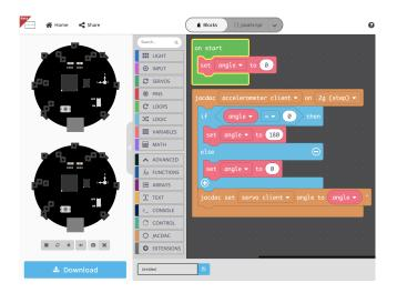
Figure 5: The customised MakeCode programming environment for Brookdale. A program that changes the rotation of a Motor Bead when a step is detected by a Motion Bead.
